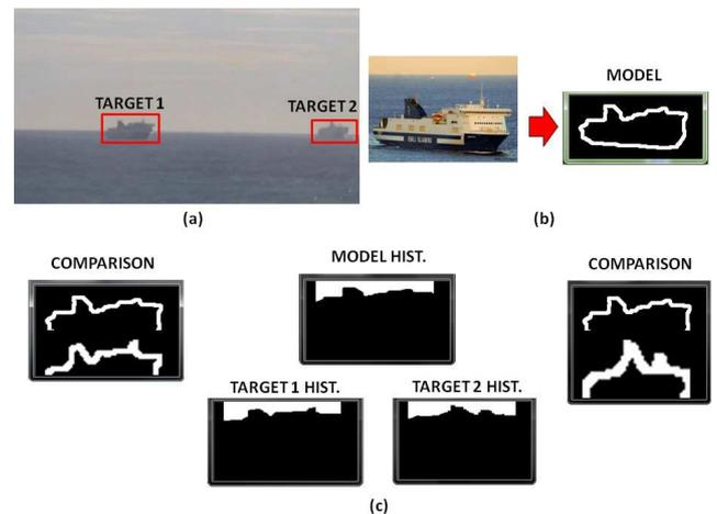
Figure 7. Target silhouettes extraction and comparison.
